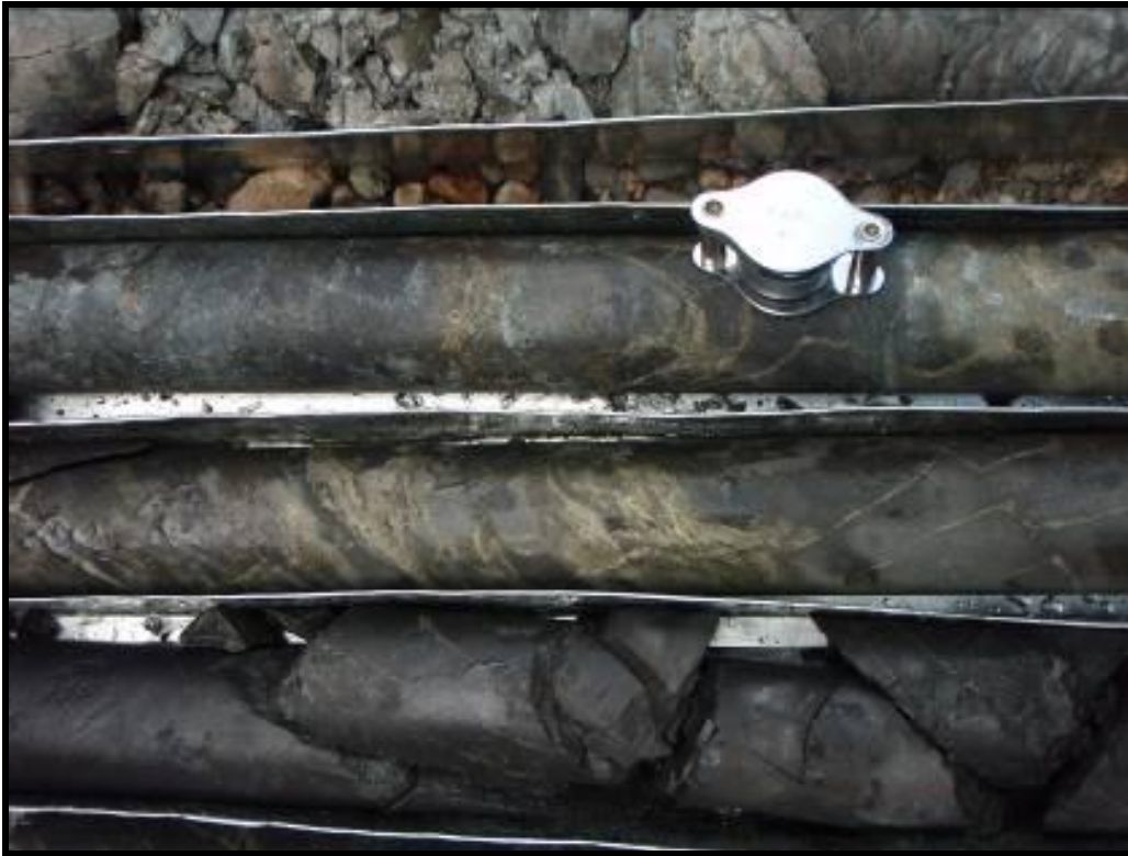
Figure 4 – TGD 108 - copper mineralization in porphyry skarn
