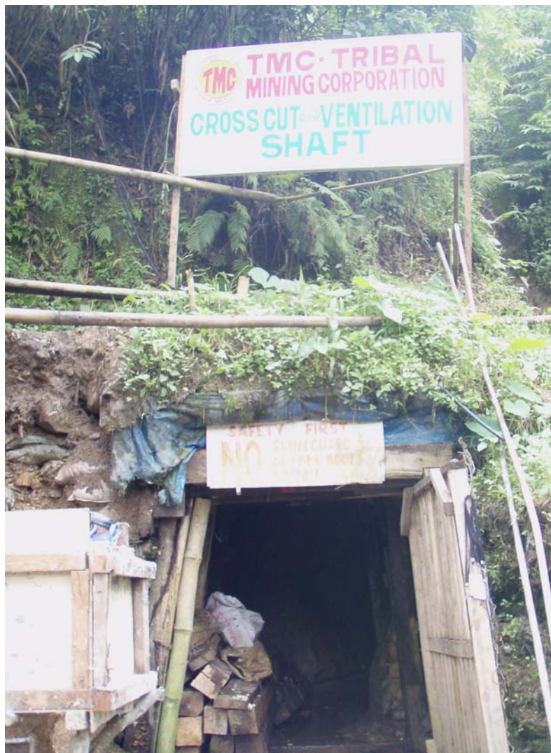
BELOW: The ventilation and alternative egress shaft which is being advanced some 100m ahead and to the east of the “Mafoko Portal” of the decline face. This shaft is being sunk on a gold lode and will provide early trial production when the advancing decline is connected.
