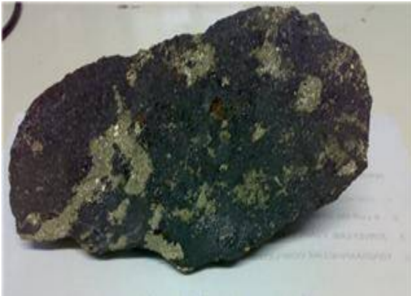
Rock from Kapanawan shows massive Magnetite with Pyrite and Chalcopyrite
