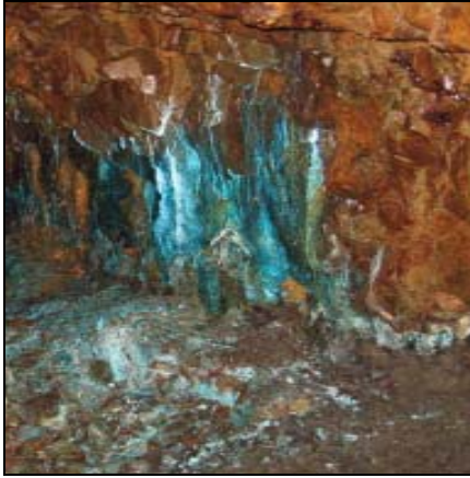
Copper oxide in K1 Adit Kalamatan Deposit
