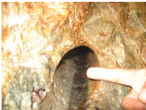
Old Diamond Drill hole observed in underground Adit
